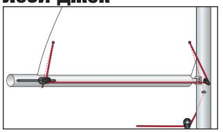
**Single Line:** The single line reefing kit is easy to install and use. To reef, simply ease the halyard to a predetermined mark and pull the single reef line taut. Ideal for boats from 22 ft to 27 ft (6.7 m to 8.2 m) with a maximum sail area of 150 ft $^2$  (14 m $^2$ ).
