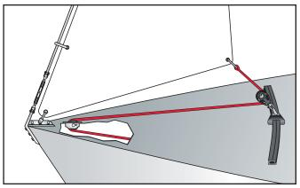
**Standard Self-tacker:** This system is often used on course racing keelboats like Solings. The traveler track is bent in a radius equal to the distance from the headstay to the sheeting point along the LP of the sail.
