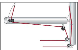
**Dual Line:** This dual-line system is common on boats 30 ft (9 m) and larger. Position blocks so line pulls down and out to keep the sail flat and prevent lateral loads on the luff rope or luff sliders.
